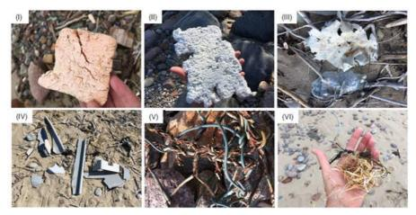
(I-II) various types of expandable polystyrene, (III) non-woven geotextile material, (IV) facing fiberglass profiles, (V) gabion mesh with plastic coating (PVC / HDPE), (VI) fragments from a textive big bag (PP).
