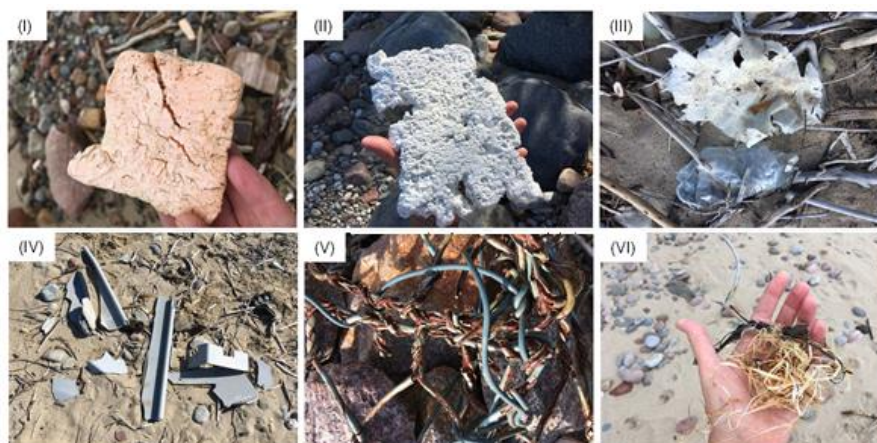
(I-II) various types of expandable polystyrene, (III) non-woven geotextile material, (IV) facing fiberglass profiles, (V) gabion mesh with plastic coating (PVC / HDPE), (VI) fragments from a textile big bag (PP).
